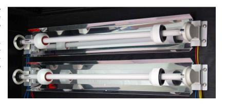
4. Place water proof endcaps at ends of reflector using wiring diagram below. Align the single holes of endcap and reflector attachment. Secure the endcaps and reflector using the sheet metal screws, first going through the endcap mount, then into the drilled holes in the reflector.
