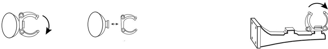
1. Remove light swivel clips from suction cups by turning 90 degrees and removing.
