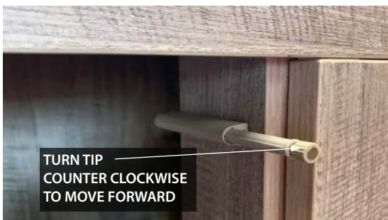
14 Adjust door open/close magnet to ensure door opens when pushed.
